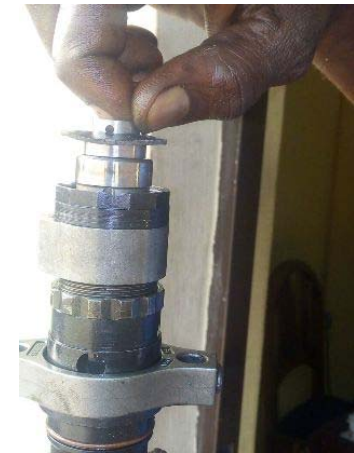
Worn out injector Typical Injector component clearances is 2 – 5 microns
