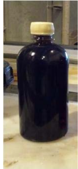
Representative sample of newly supplied Diesel Fuel; ISO Cleanliness 23/23/22
